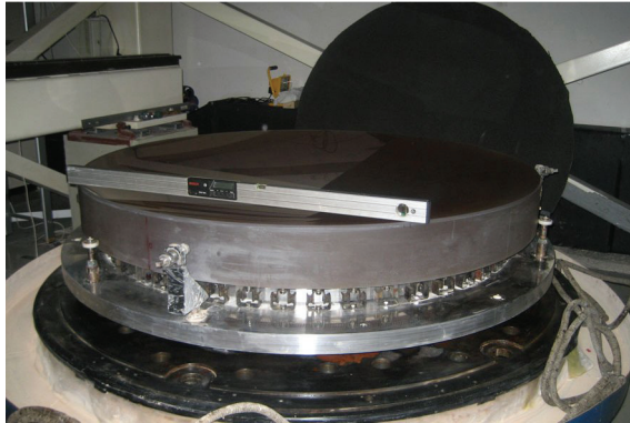
Figure 29. AM1 under test at AMOS, the manufacturer of AM1. Shown is AM1 after its spherical lapping. In its final shape, AM1 will be an 1.7-meter aspherical mirror with a standard aluminum coating.
