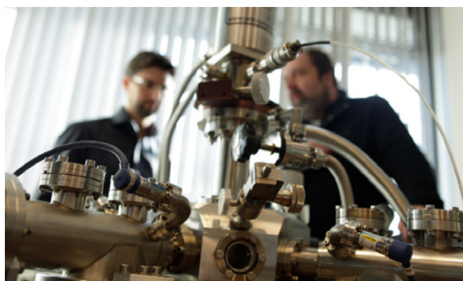
Fig. 1: SURFRESIDE2, a sophisticated cryogenic ultra-high vacuum setup in which atoms impacting on an interstellar ice analogue are used to increase molecular complexity in the solid state.
