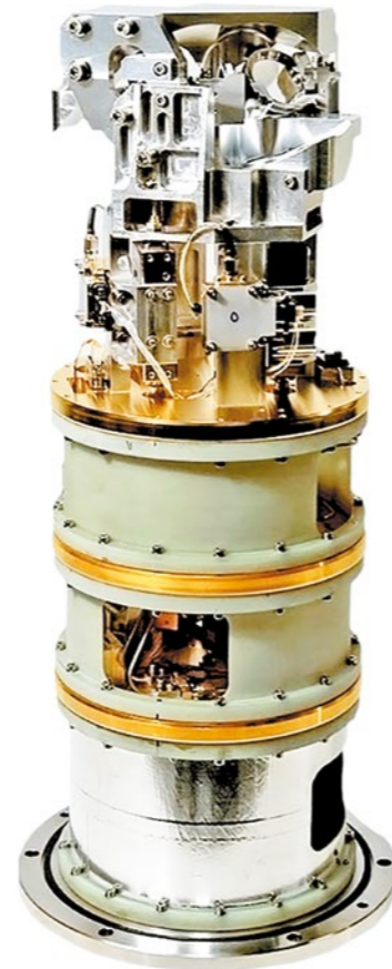
Figure 1: SEPIA660 (ALMA Band 9) cartridge, from Baryshev et al. (2015).
