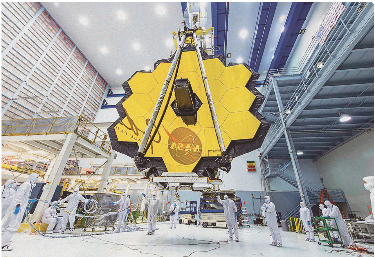
NASA technicians lift the James Webb Telescope, using a crane, and move it inside a clean room at NASA's Goddard Space Flight Center in Greenbelt, Maryland. The scientific successor to NASA's Hubble Space Telescope, Webb is the most powerful space telescope ever built. Credits: NASA/Desiree Stover
