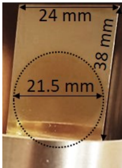
Figure 2.9: The darker circle, outlined by a dashed circle, is carbon deposit that resulted from the atomic beam on the gold surface of the substrate. The entire beam is on the flat surface, and the angle at which the picture is taken makes it appear that the lower part is clipped. A beam diameter of 21.5 mm is measured on a sample plate that has a size of 38 mm \times 24 mm. Note that contrast has been added to the image to visualize the area with impacting C-atoms.
