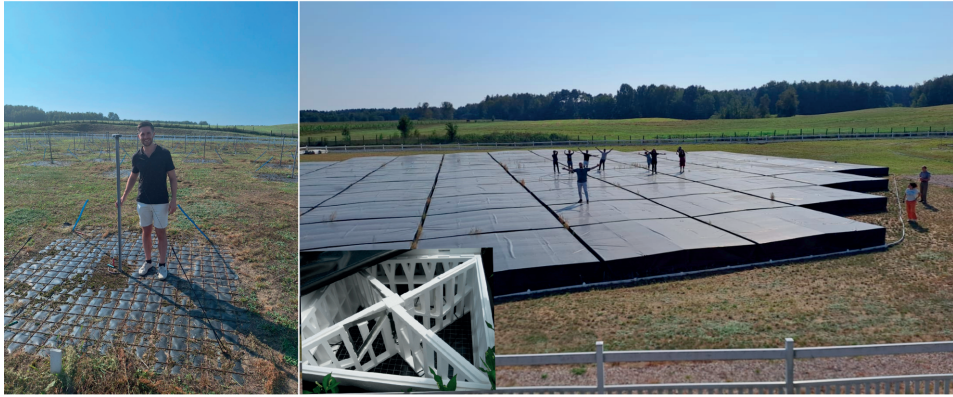
Figure IV: Different LOFAR antennas. On the left, a low-band antenna is shown with a human for scale. In the middle below, an image of a high-band antenna is displayed, which is concealed beneath the tiles on the right, with humans standing on top for scale. These pictures were taken at the PL612 station in Baldy (Poland) by the author and his colleagues.
