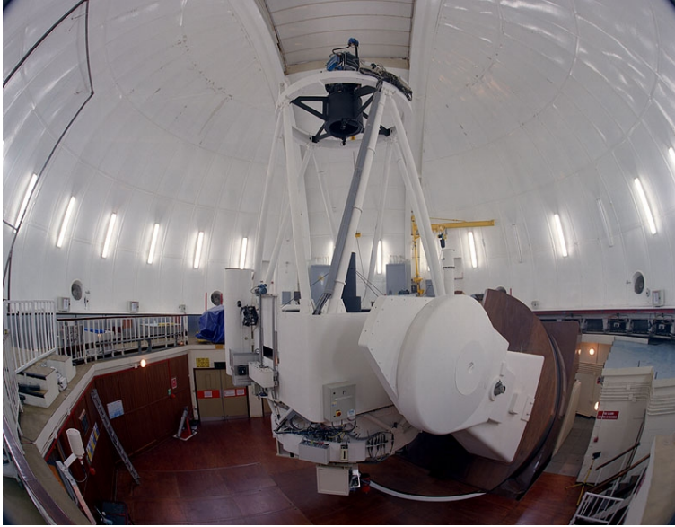
Figure 1.6: The 2.5m Isaac Newton Telescope in its dome on Observatorio Roque de los Muchachos on La Palma. The telescope has an equatorial mount designed for its initial location in the UK and modifications had been made in order to use the telescope at lower latitudes. The Wide Field Camera is mounted on the prime focus and cooled by liquid nitrogen. Credit: Isaac Newton Group.
