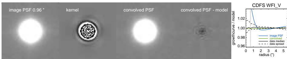
Figure 2.25: Example of a case where the original PSF was worse than the target PSF. See Figure 2.24 for a description of the panels. Here the image was deconvolved . A small residual is left after subtracting the model PSF from the deconvolved PSF, but the integrated flux at r = 0.6'' corresponds well, to within 1%.
